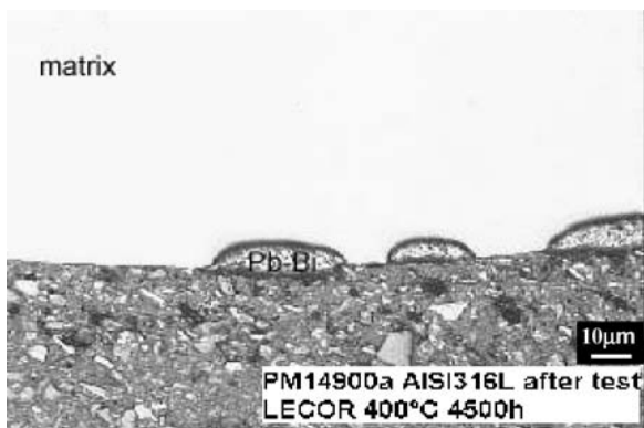
Figure 3 Optical micrograph of austenitic steel exposed in LECOR loop after 4500 h ( C_{[O_2]} = 10^{-8} - 10^{-10} wt%, T = 400^\circ\text{C} ).
